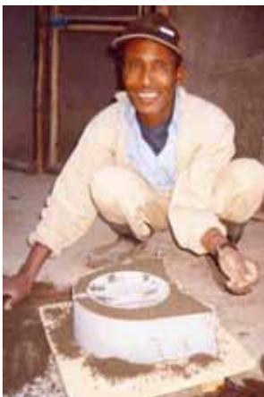
trainee using a mould to make a stove flue
